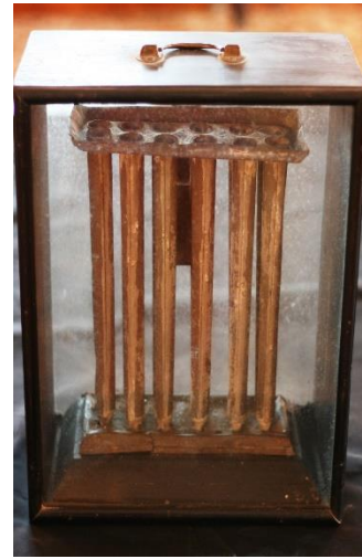
In Galveston's earliest days, residents had to rely on candles to light their homes at night. Candles were handmade in tin molds like this one. (Library purchase)
